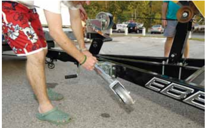
Fold up the front wheel assembly.
