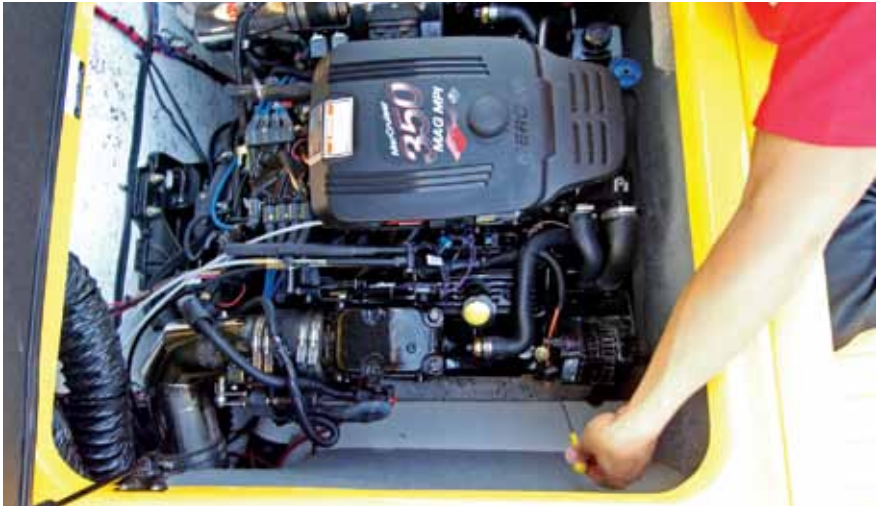
Pull the dipstick to check the engine fluid levels.
