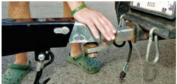
Fold down the hitch locking mechanism.
