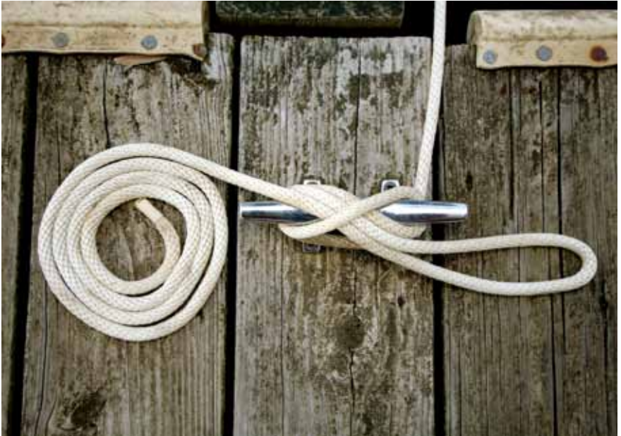
Neat and efficient figure eights on a cleat with slippery hitch and coil
