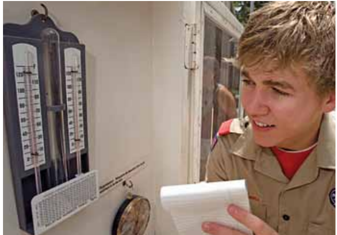
By noting changes in relative humidity as indicated on a hygrometer, you can determine whether the day will be muggy or comfortable.
