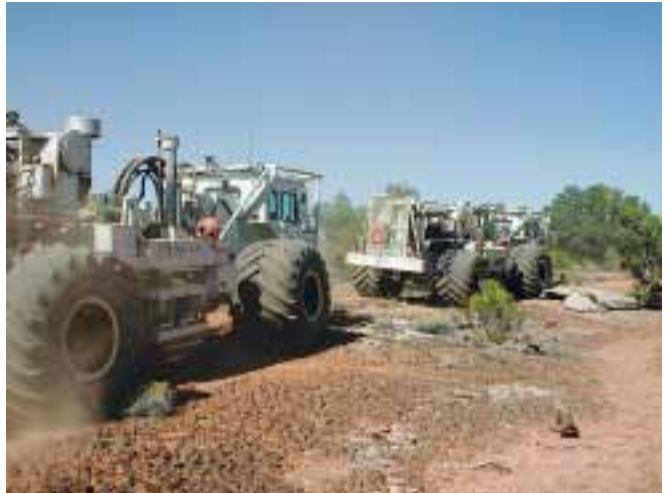
Seismic trucks generate energy waves into Earth to help scientists record reflections against the different rock layers.
